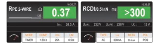
2-wire continuity test
