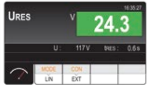
Residual voltage measurement
