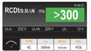
Test on RCDs
