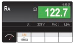
Measurement of non-trip earth resistance
