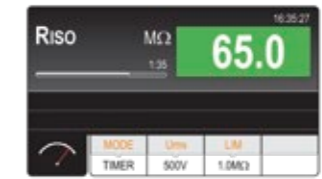
Measurement of insulation resistance
