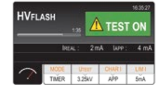
Dielectric strength test
