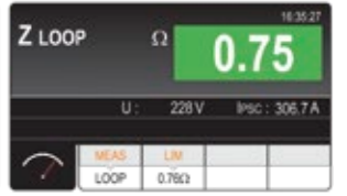
Measurement of Loop impedance
