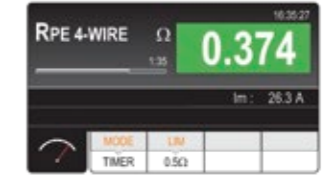
4-wire continuity test
